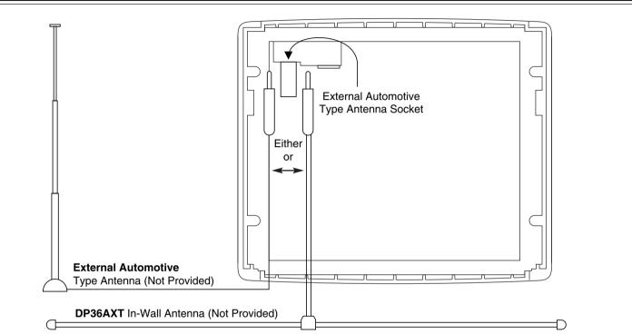
The LS3500CD have a provision for a standard automotive antenna. If an automotive antenna is used, plug the male plug from the antenna into the female receptacle provided on the unit. If an automotive antenna is not available or is undesired, we recommend the use of a Magnadyne DP36AXT di-pole antenna substitute. Plug the male plug from the DP36AXT into the female receptacle of the LS3500CD unit and allow the cable of the antenna to lay inside the wall.
